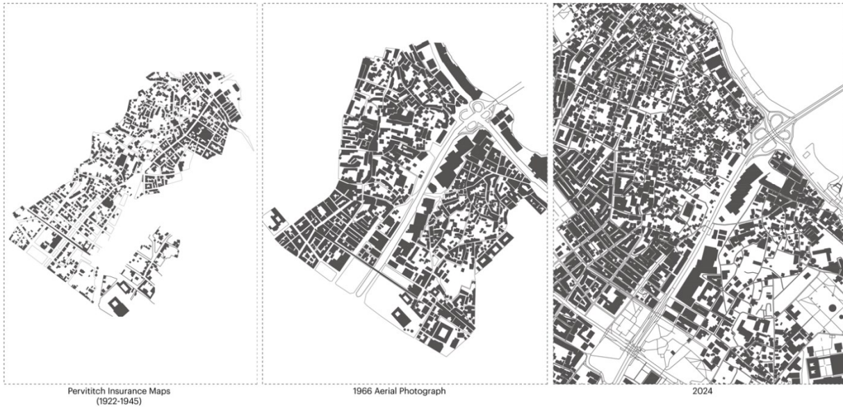
Figure 6. The changes in building fabric between Pervititch Insurance Maps (1922-1945) and 2024 maps.
