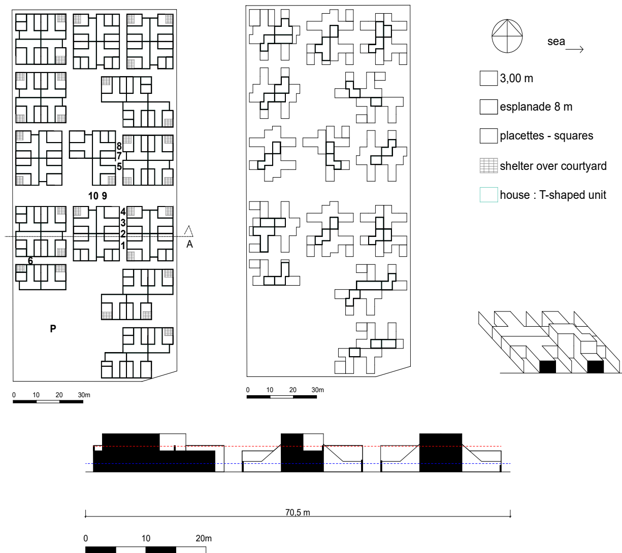
Figure 2. Village Grec. Left: Ground floor with pedestrian street widths and SVF locations; Middle: first floor Right: schematic diagram of the assembled "T" units Bottom: Section A. Red line: mean building height; Blue line: Absolute Rugosity or mean urban canopy height
