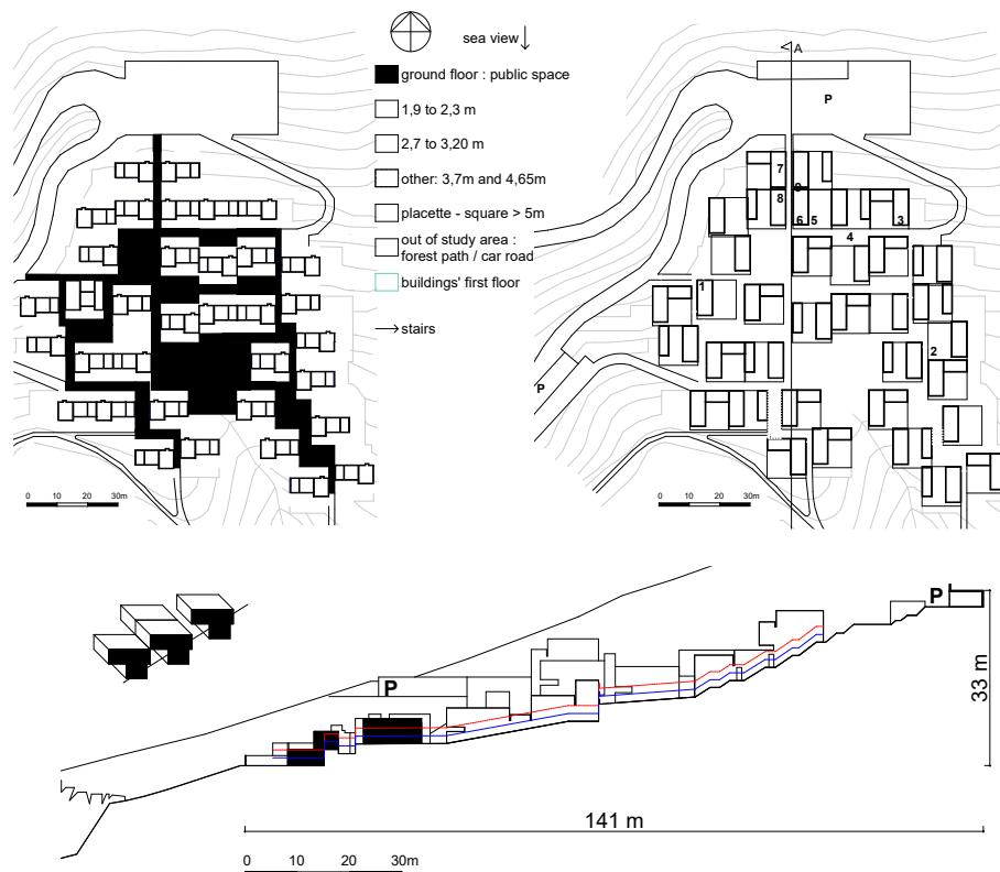
Figure 5. Merlier. Left: ground floor: partial underground units, public pedestrian space in black Right: first-floor plan: pedestrian street widths and SVF locations Bottom left: schematic diagram of the grid assembly of units on a slope; Bottom right: Section A. Red line: mean building height; Blue line: Absolute Rugosity or mean urban canopy height
