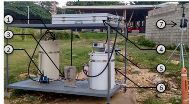
Figure 3. Experimental bank: 1. Water reservoir, 2. Pump, 3. Rotameter, 4. Solar collector, 5. Data acquisition unit, 6. Water reception tank, 7. Weather station.
