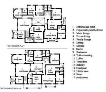
Figure 9. Plan of a Contemporary Hausa Building Designed by Zailani and Sa'ad Raji (Aliyu, 2015).
